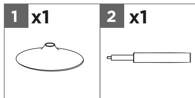
Remove the cap on top of gas lift **2** before assembly. Place the gas lift **2** into the hole in base **1**.
