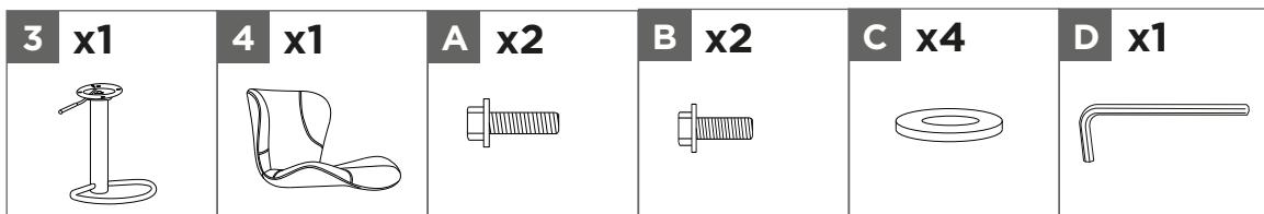
Align the holes of the seat plate **3** to the base of the seat **4**. Connect using the screws **A** in the front and **B** in the back with washers **C**. Tighten with hex key **D**.
