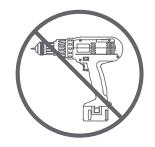
NOTE: To avoid damage, ensure screws are hand tightened. DO NOT USE POWER TOOLS TO ASSEMBLE YOUR UNIT.
