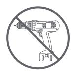
To avoid damage, ensure screws are hand tightened. DO NOT USE POWER TOOLS TO ASSEMBLE YOUR UNIT.
