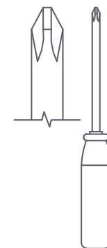
No. 2 Phillips Screwdriver Tip Shown Actual Size
