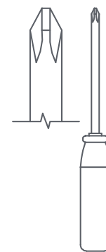
No. 2 Phillips Screwdriver Tip Shown Actual Size
