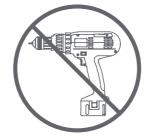
To avoid damage, ensure screws are hand tightened. DO NOT USE POWER TOOLS TO ASSEMBLE YOUR UNIT.
