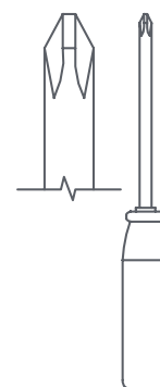
No. 2 Phillips Screwdriver Tip Shown Actual Size
