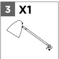
Pull the excess cord from the base **1**, and insert and thread the arm assembly **3** onto tube **2 (d)** by turning clockwise until secure.
