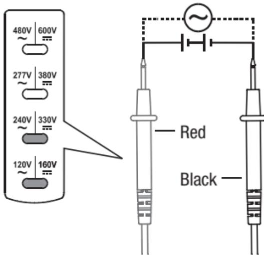
1. Connect the red test lead and the black test lead across the voltage source or circuit to be measured.
