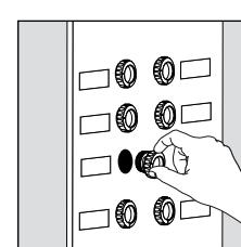
**NOTE:** Shutting off a wall switch that controls the light is not sufficient to prevent electric shock.
