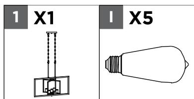
Install 5 E26 medium base bulbs 1 into the sockets of the fixture 1.
