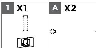
Thread the wires through one of the rods **A**, and twist the rods clockwise into the threaded stems of the fixture **1** until they are secure.
