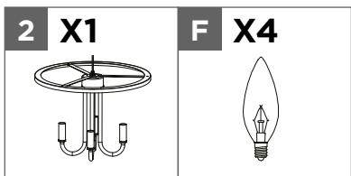
Install four E12 candelabra 40 watt bulbs **F** (not included) onto light fixture **2**.
