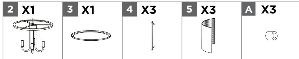
Place the metal clip arms **4** on the metal ring **3** with metal clips **4** facing inward and secure from below with decorative nuts **A**. Carefully place glass panels **5** one at a time onto the metal ring **3** and into the metal clip arms **4**.
