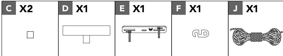
Cut the cord (J) to the desired length (optional). When cutting the cord, ensure that the length needed for the strain relief buckle is accounted for.
