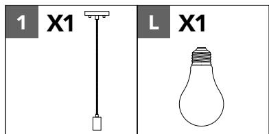
Insert and screw the light bulb (L) into the socket of the fixture (1). Use one medium base (E26), 60 W max bulb
