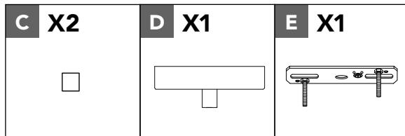
Align the mounting holes on the canopy (**D**) with mounting screws on the mounting bracket (**E**).
