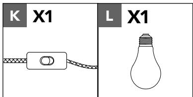
Insert and screw the light bulb (L) into the socket. Use one medium base (E26), 60 W max bulb.
