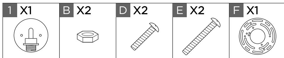
Thread the fixture screws **E** into the holes of the mounting bracket **F**.
