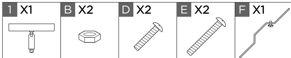
Thread the fixture screws **E** into the provided holes of the mounting bracket **F**.
