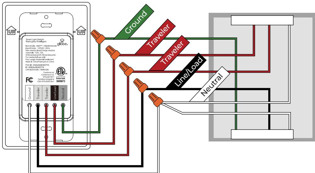
Ground (Optional. The ground wire is suggested to be connected up).
