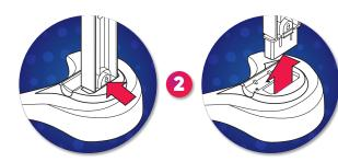
Push the release lever at the base of the device stand post and lift up to remove the device stand post from the base.
