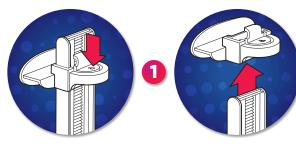
Press the release lever on the back of the device stand clip, then slide the clip up and off the device stand post.
