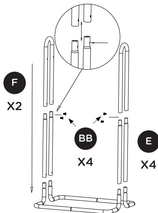
**STOP** - Ensure the screw holes are aligned on the inside.
