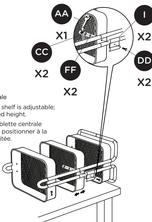
**STOP** - Assemble one side at a time with product on its side.
