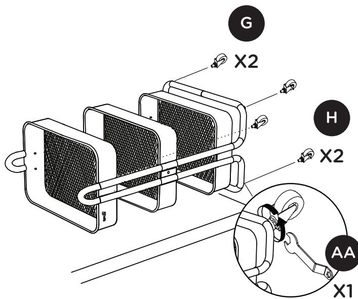
**STOP** - Ensure locking wheels are on the same side (both on one short side or both in the front).
