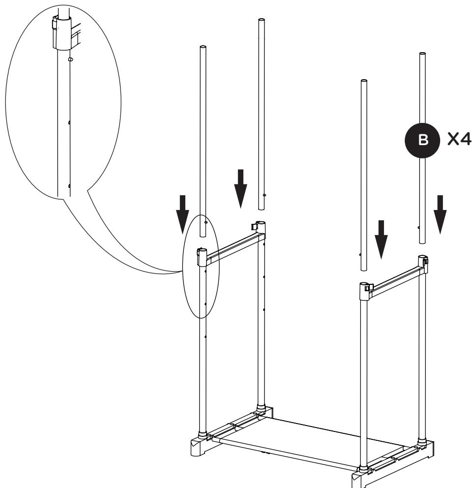
**STOP** - There are 3 holes on one end of part C to adjust rack to your desired height.
