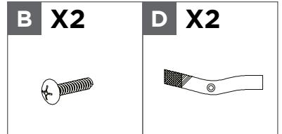
Secure the strap **D** to the wall using the bolt **B** at marked stud or wood locations.
