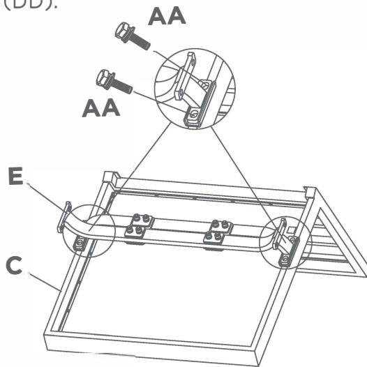
**NOTE:** Do not completely tighten.
