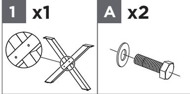
Connect the right leg frame **1** to the assembled frame using the screws **A** with washer, aligning the holes.
