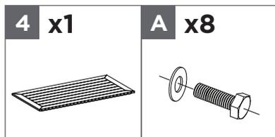
Connect the table top **4** to the assembled frame using the screws **A** with washer, aligning the holes.
