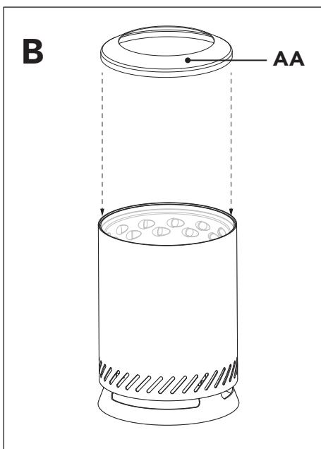
**Step 2:** Position the flame ring (AA) as shown. This will direct the flame upwards for the best secondary burn (see image B).
