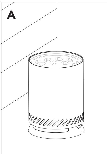
**Step 1:** Position the firepit on a level surface. If using pellets, insert the pellet adaptor (see image A).
