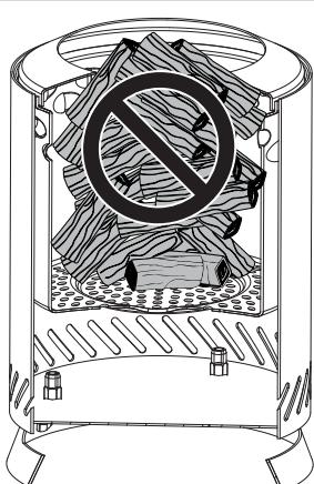
Never stack wood higher than the interior burn holes. Doing so will cut off airflow and cause your fire to smoke. Make sure wood is resting under the holes and that they are clearly visible after fuelling (see image D).
