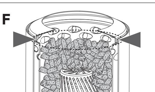
**Step 2:** Add pellets to the burn chamber. Do not overfill; pellets should not be higher than the interior burn holes (see image F), as this can obstruct airflow and cause the fire to smoke.
