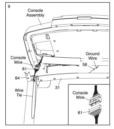
Set the console assembly on the Right and Left Handrails (84, 85). Make sure that no wires are pinched. Insert the excess Upright Wire (81) into the Right Upright (90).
