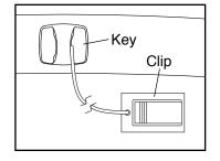
will light. IMPORTANT: In an emergency, the key can be pulled from the console, causing the walking belt to slow to a stop. Test the clip by carefully taking a few steps backward; if the key is not pulled from the console, adjust the position of the clip.
