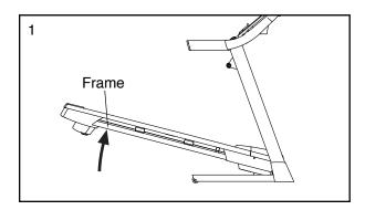
Hold the frame firmly with your right hand. Pull the latch knob to the left and hold it. Raise the frame until the latch plate is past the latch pin. Then, slowly release the latch knob; make sure that the latch plate is resting against the latch pin.
