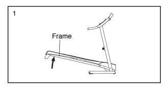
Hold the treadmill firmly with your right hand as shown. Pull the latch knob to the left and hold it. Raise the frame until the latch plate is past the latch pin. Then, slowly release the latch knob; make sure that the catch is resting against the latch plate.
