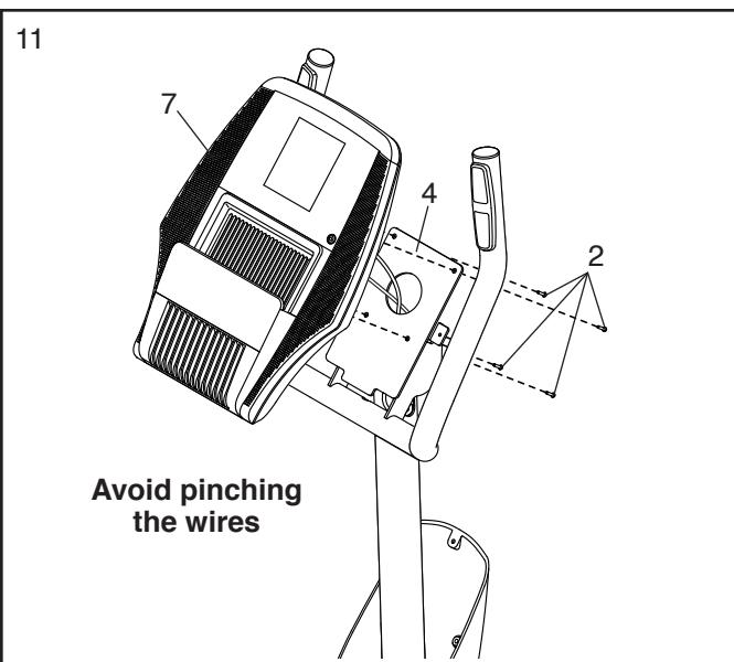
12. Slide the Console Cover (3) upward to the Handlebar (4). Attach the Console Cover to the Handlebar and to the Console (7) with three M4 x 16mm Screws (2); **start all the Screws, and then tighten them.**
