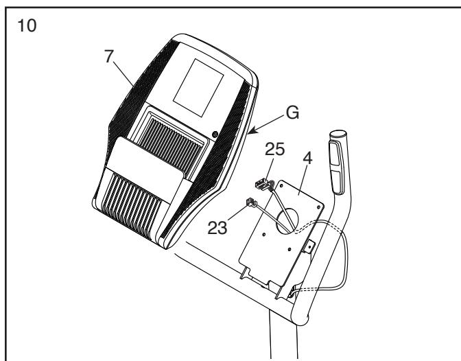
11. **Tip: Avoid pinching the wires.** Attach the Console (7) to the Handlebar (4) with four M4 x 16mm Screws (2); **start all the Screws, and then tighten them.**
