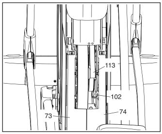
When you have properly adjusted the drive belt, reattach the rear shield and press the shield cover onto the rear shield.
