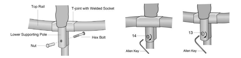
• Repeat the steps above to attach all six Supporting Poles onto the vertical legs of the trampoline.
