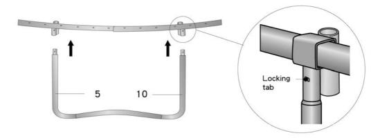
• After completing the assembly, the trampoline frame should look like the illustration below.
