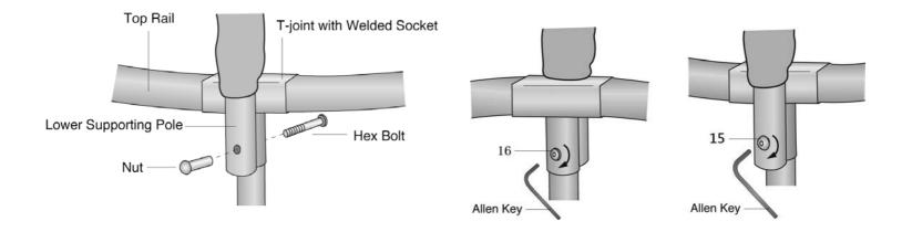
• Repeat the steps above to attach all six Supporting Poles onto the vertical legs of the trampoline.
