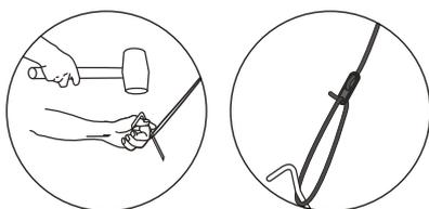
**Tent must be completely guyed out to prevent rain water from pooling on the roof/fly causing frame damage.**
