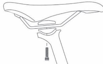
Micro-adjust seat post with integrated clamp
