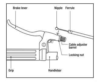
**CAUTION:** If the barrel adjuster is loosened too much it may fall out, causing brake failure.
