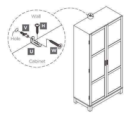
Drill a 3/16" (5 mm) diameter hole in the wall. Tap the wall anchor (  $\vee$  ) into the hole until it is flush.
