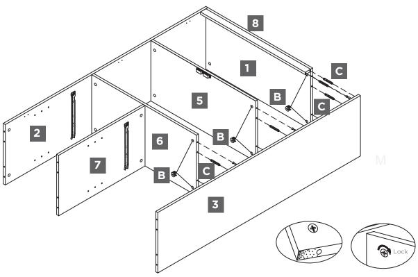
Proper orientation of cam lock.
