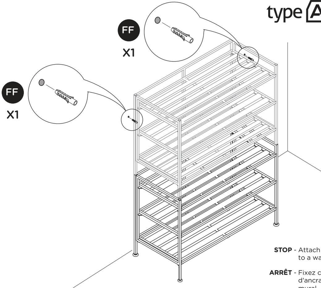
**STOP** - Attach anchors (FF) to a wall stud.
