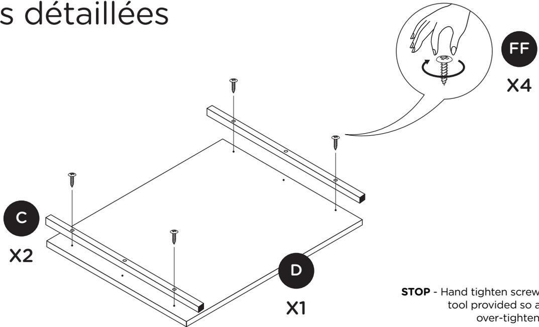
**STOP** - Hand tighten screws or use tool provided so as not to over-tighten screws.
