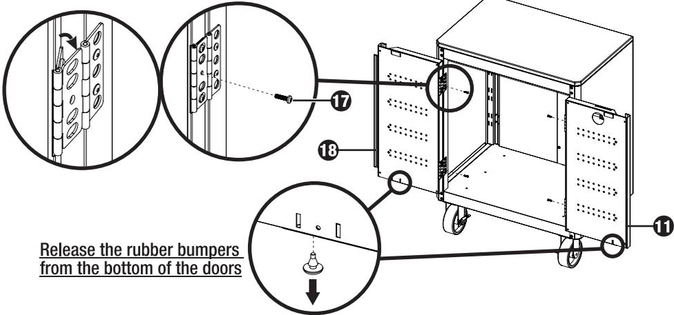
Release the rubber bumpers from the bottom of the doors
