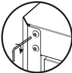
Tighten all screws you previously tightened by hand
