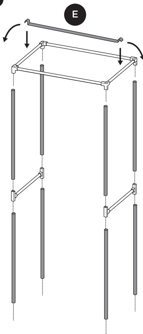
**STOP** - Place the ends of the hanging rail (E) on the side support bars and press down to snap into place.
