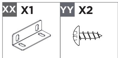
Put the insert into place. Secure the insert by using Bracket (XX) and fasten the Bracket to insert by two Screws (YY).
