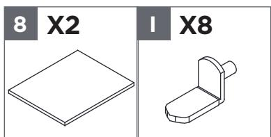
Insert eight Shelf Pins (I) into the holes in the side compartment as shown, then place the Adjustable Shelves (8) onto the Shelf Pins.
