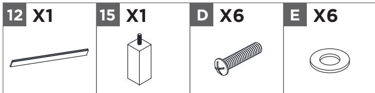
Attach Bottom Trim (12) in place using six Washers (E) and six Bolts (D). Attach Foot (15) in place by securing the pre-attached Screw into the designated hole in the Bottom (11).
