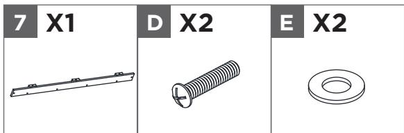
Attach Top Trim (7) in place by using two Washers (E) and two Bolts (D).
