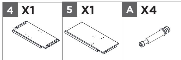
Securely screw four Cam Bolts (A) into the designated holes of Left Divider (4) and Right Divider (5).
