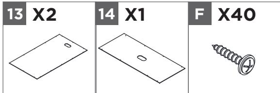
Align and attach Back Panels (13) and Middle Back Panel (14) in place by using forty Screws (F).
