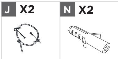
Follow the instructions printed on the plastic bag containing the tipping restraint hardware to attach the Anti-tipping Hardware (J) to the unit and the wall.
