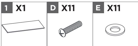
Align and attach Top (1) in place by using eleven Washers (E) and eleven Bolts (D).
