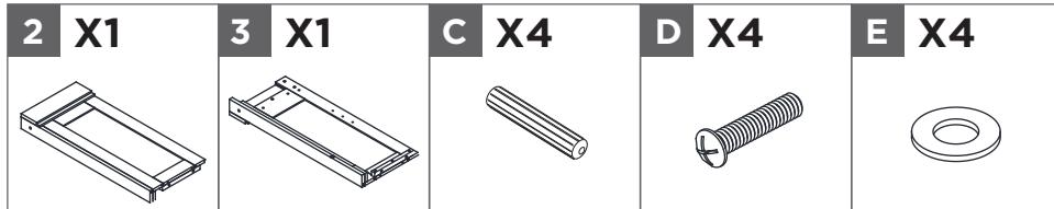
Attach Left Side Frame (2) and Right Side Frame (3) to Bottom (11) by using four Wood Dowels (C), four Washers (E) and four Bolts (D).
