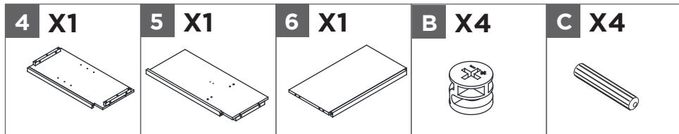
Attach Left Divider (4) and Right Divider (5) to Fixed Shelf (6) by four Wood Dowels (C) and engaging four Cam Locks (B).
