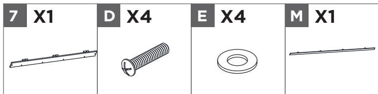
Attach Slide Bar (M) to Top Trim (7) by using four Washers (E) and four Bolts (D).
