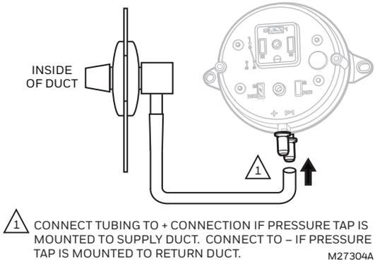
**Fig. 11. Install tubing.**
