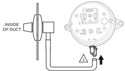
**⚠** CONNECT TUBING TO + CONNECTION IF PRESSURE TAP IS MOUNTED TO SUPPLY DUCT. CONNECT TO - IF PRESSURE TAP IS MOUNTED TO RETURN DUCT.
