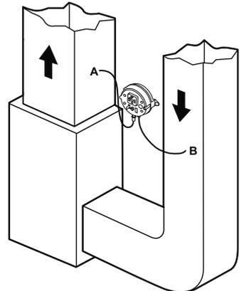
**SUPPLY DUCT INSTALL** - AIR LINE ONLY TO TAP A, CONNECTED TO THE + PORT ON THE AIR FLOW SWITCH
