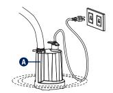
**NOTE:** Make certain you unwind the garden hose completely. Kinks in the hose will restrict the pump, preventing it from priming, which is the first step to pumping water. The water level must be at 1" (2.5 cm) for the pump to prime and operate.
