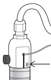
3. Loosen the connector cover screw & remove the cover and **wait 10 minutes for the lamp to cool.**
