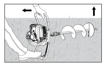
6. Holding the unit firmly, pull the recoil starter grip 2 times to prime with fuel, then pull until engine starts. Use short pulls and do not allow the rope to snap back. Do not pull more than 6 times.
