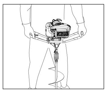
8. After the engine runs for 10-15 seconds, move the choke lever to the "RUN" position.
