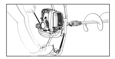
7. Once the engine starts, stand the auger up in the vertical position and allow to run for 10-15 seconds.
