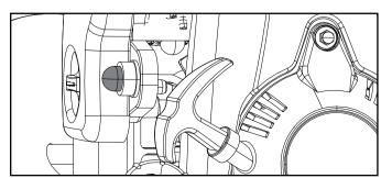
4. Set the choke lever to the "CHOKE" position.
