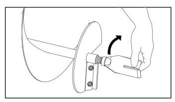
2. To tighten securely, grasp the auger bit shaft with one hand while placing an adjustable wrench on the fishtail bit point and tighten until it is securely in place.
