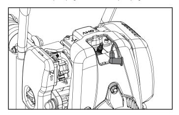
3. Use a spark plug socket tool, or a 41/64 in. (16 mm) socket to remove the plug.
