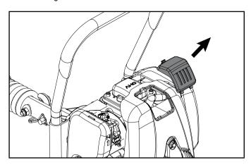
2. Remove the spark plug cable from the spark plug.
