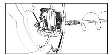
6. Once the engine starts, stand the auger up in the vertical position.
