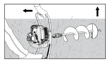
Holding the unit firmly, pull the recoil starter grip until engine starts. Use short pulls and do not allow the rope to snap back.
