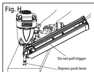
(3) With finger off the trigger, depress the push lever against the workpiece (Fig. I).
