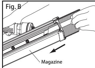
2. Insert nail strip into the back of the magazine (Fig. B).
