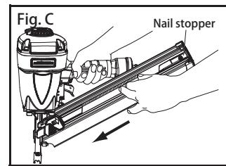
3. Slide the nail strip forward in the magazine. The nail strip should pass the nail stopper (Fig. C).
