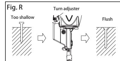
When the adjuster is released it will spring back up and can be set with a click at each 1/4 rotation. The adjuster changes the nailing depth approximately 0.25 mm per 1/4 rotation.
