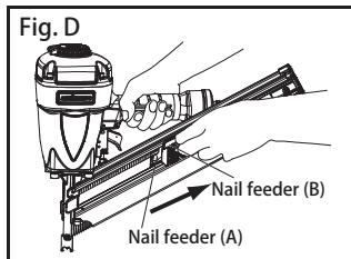
4. Pull the nail feeder (B) back to engage the nail feeder (A) on the nail strip (Fig. D).
