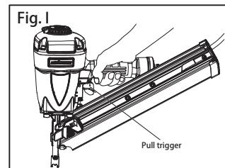
(4) Without touching the trigger, depress the push lever against the workpiece. Pull the trigger.
