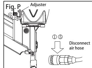
2a. If the nails are driven too deep, pull the adjuster downward and turn clockwise (Fig. Q).
