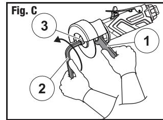
2. Insert the hex bolt (1) upon fixing the new cutting disc (2) in position (Fig. D).
