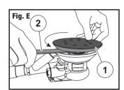
3. Place the new sanding pad (1) over the nut (2) (Fig. F).
