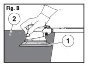
2. Place the sanding pad (1) of the sander over the workpiece (2) to be sanded (Fig. B).
