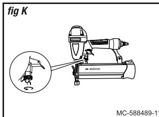
Note: If the fastener is not going deep enough, adjust the pressure of the regulator accordingly.
