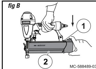
3. Insert a strip of fasteners (1) into the magazine. Ensure the points of the fasteners are facing down. Slide the pusher (2) against the fasteners to close the magazine until it comes into contact with the fasteners and locks into place (fig C). → (see nail type icon on page 19)
