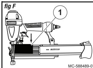
3. 7/32 Narrow Crown Staples: Insert the staples (1) from the top area of the magazine with one arm of the staple in the centre slot of the magazine and the other arm along the left side of the magazine (*fig G*).
