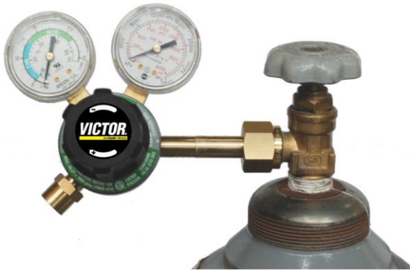
Figure 4-4: Regulator to cylinder valve
