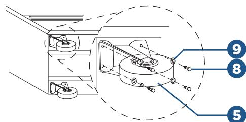
Carefully lay the cabinet on its back with a soft mat underneath for protection. Position the two rigid castors (5) on one side of the bottom of the cabinet. Insert the M8 x 25 hex bolts (8) through washers (9), then through the castors and into the bottom of the cabinet. Tighten securely.
