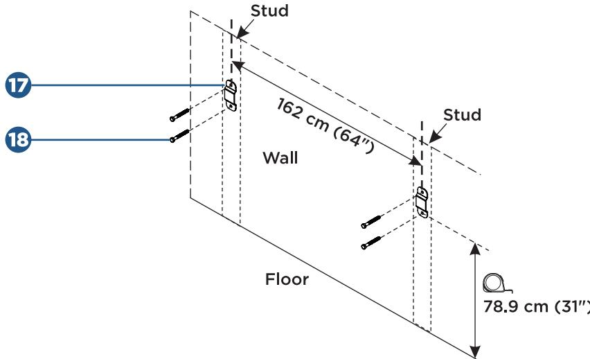
Install another two safety brackets (17) to both sides of the cabinet with four M6 x 12 hex bolts (14). Tighten securely.
