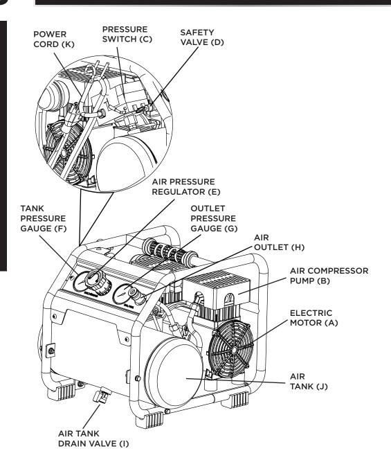
A. ELECTRIC MOTOR: The motor is used to power the pump. It is equipped with a thermal overload protector. If the motor overheats for any reason, the thermal overload protector will shut it down in order to prevent the motor from being damaged.
