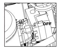
2. Open the tank drain valve (I) by turning it counter-clockwise to permit the air to escape and prevent air pressure build-up in the air tank during the break-in period.
