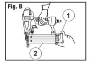
Hold the air-powered brad nailer firmly with one hand, and use the other hand to press the latch (1) on the magazine (2) and slide it back (Fig. B).
