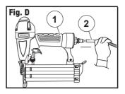
4. Plug in compressor, turn it on, set the pressure regulator to 90 PSI (6.2 bar), and attach one end of the air hose to the compressor and the other end of the air hose (1) to the tool (2). Use plumber's tape to prevent air leaks (Fig. D).
